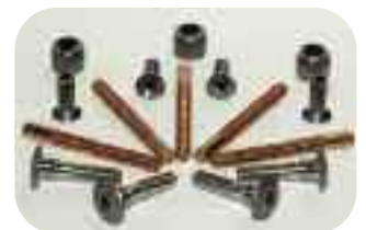
Fig. 3 — Cold-forged parts produced from various standard materials.
