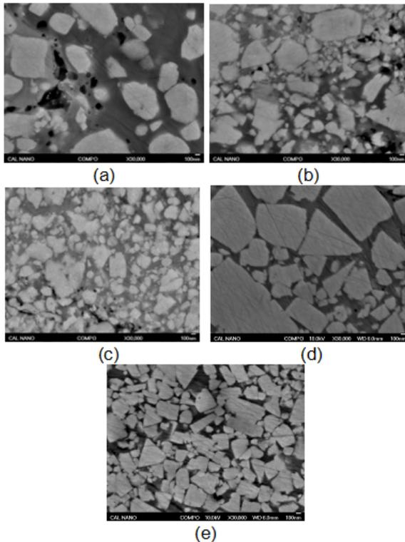
**Figures 3a, b, c, d and e:** High resolution (30,000x) SEM images of cross-sectioned thermal spray coatings showing the WC grains: (a) Coating A (commercial powder); (b) Coating B; (c) Coating C; (d) Coating E; and (e) Coating F
