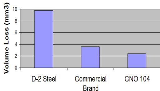
**Fig. 4:** Wet Abrasion Wear Testing, G105-02
