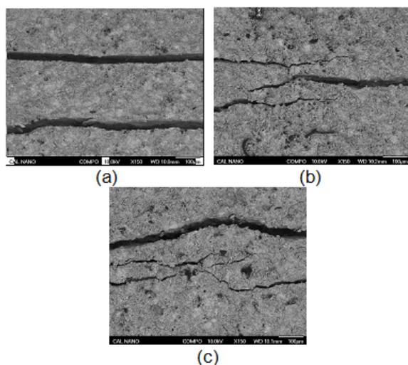
**Figures 5a, b and c:** SEM images (150x) of bend test samples showing coating cracks: (a) Coating A (commercial powder); (b) Coating B; (c) Coating C
