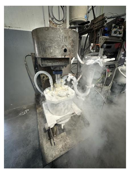
Two cryomills in operation, breaking down metal or polymer materials into fine particles
