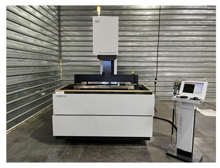
Cutting edge molybdenum EDM wire machine to assist with post-processing of customer parts
